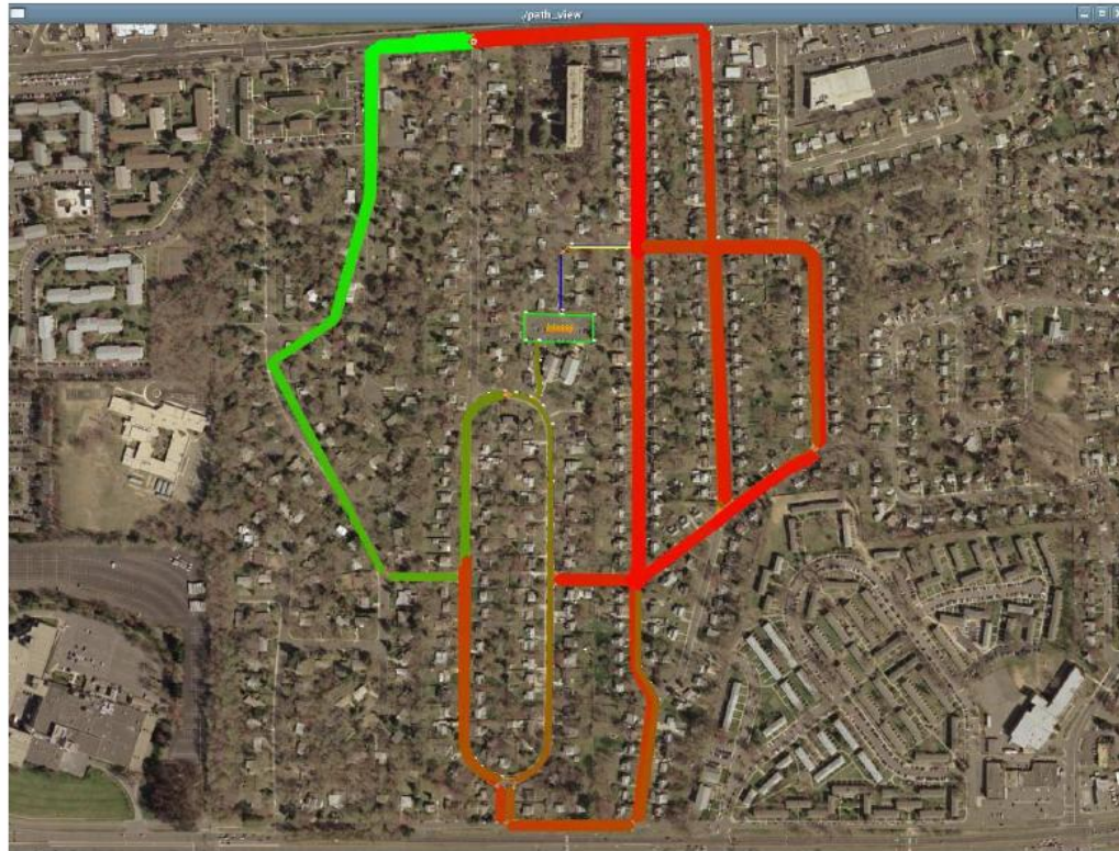
Figure 12: Global planning: Dynamic programming propagates values through a crude discrete version of the environment map. The color of the RNDF is representative of the cost to move to the goal from each position in the graph. Low costs are green and high costs are red.
