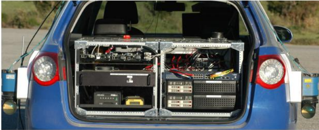
Figure 2: All computing and power equipment is placed in the trunk of the vehicle. Two Intel quad core computers (bottom right) run the bulk of all vehicle software. Other modules in the trunk rack include a power server for selectively powering individual vehicle components, and various modules concerned with drive-by-wire and GPS navigation. A 6 DOF inertial measurement unit is also mounted in the trunk of the vehicle, near the rear axle.
